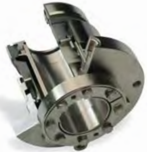
HRK-D Double seal, cartridge version, for buffer pressure or quench operation, suitable for pressure reversal (does not open if the buffer pressure fails); can alternatively be used with pumping screw to increase the circulated volume.
