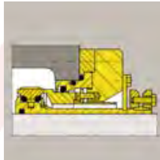
HR3 ... Single seal, cartridge version.
