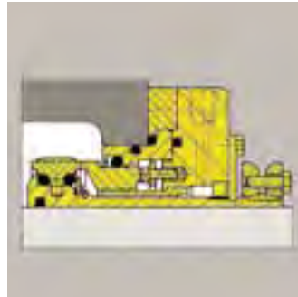
HR2 ... Single seal, cartridge version, for use with quench.
